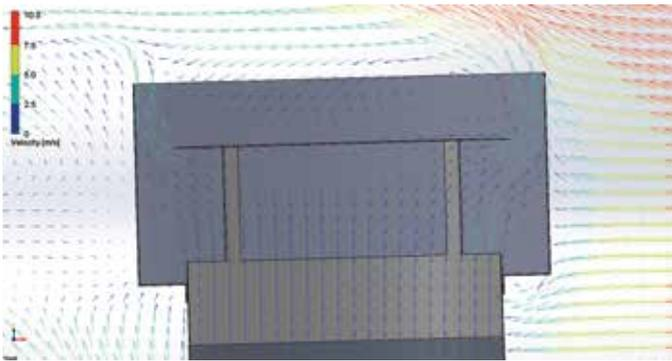
Figure 5: Velocity vectors indicating the recirculation of airflow which limits the induced flow occurring in PT2.
