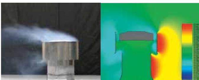
Figure 7: Comparison of smoke visualisation test and pressure contours from the CFD results occurring in PT4.
