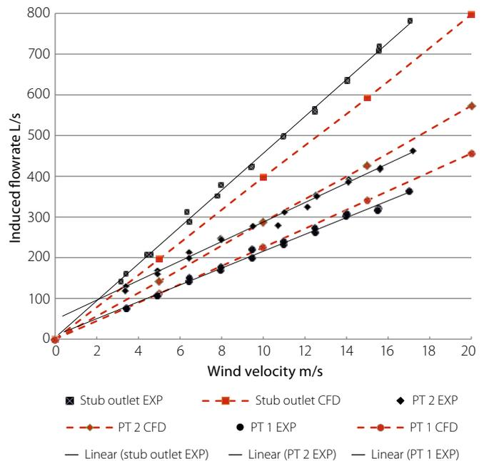
Figure 3: Preliminary comparison of experimental and CFD results of open jet wind tunnel arrangement.
