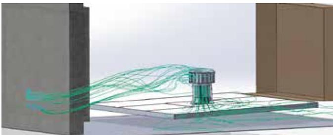
Figure 2: Virtual wind tunnel facsimile of open jet wind tunnel arrangement.
