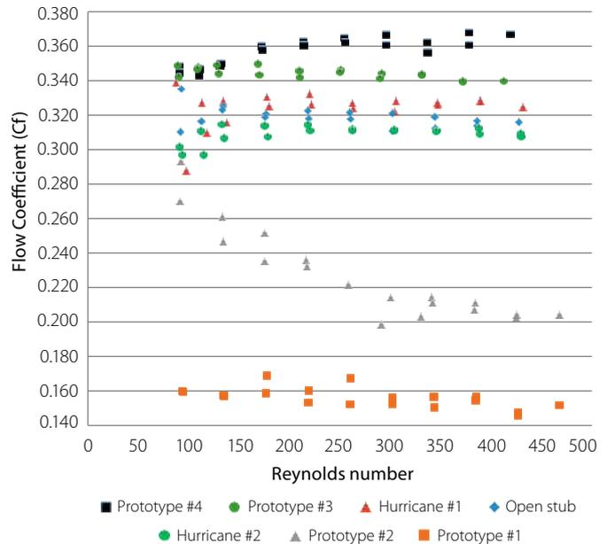
Figure 8: Comparison of ventilator induced flow performance test results.
