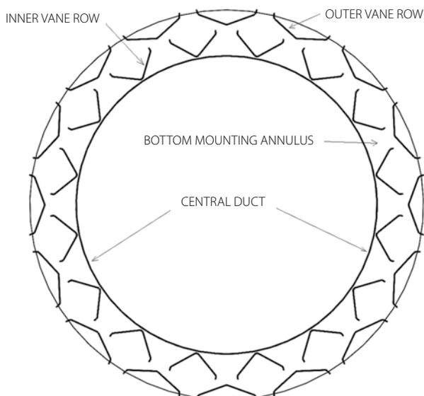
Figure 4: Plan view cross section of the vane elements arranged in a circular array with an outer row and an inner row to comprise PT1.
