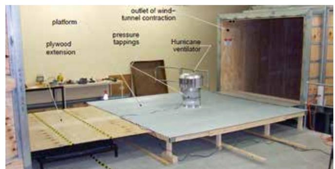
Figure 1: Open jet wind tunnel arrangement. Note that the flow is from right to left.
