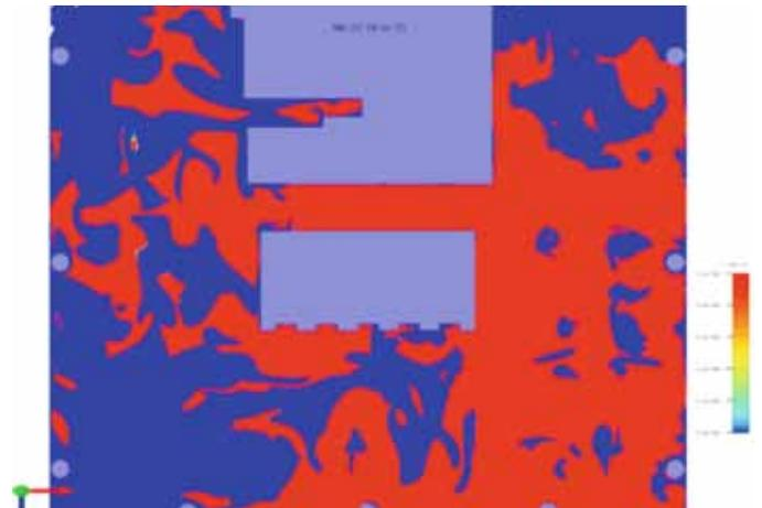
Figure 7: ACE at 2000mm height at maximum diffuser flow rates
