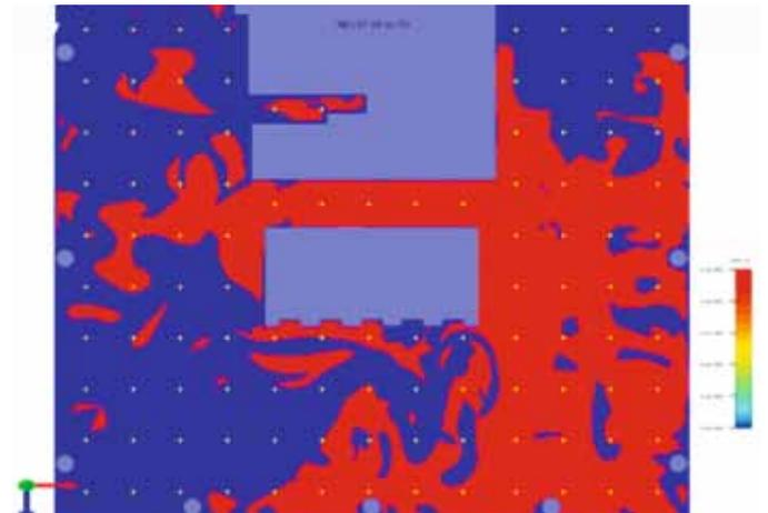
Figure 6: ACE at 1000mm height at maximum diffuser flow rates
