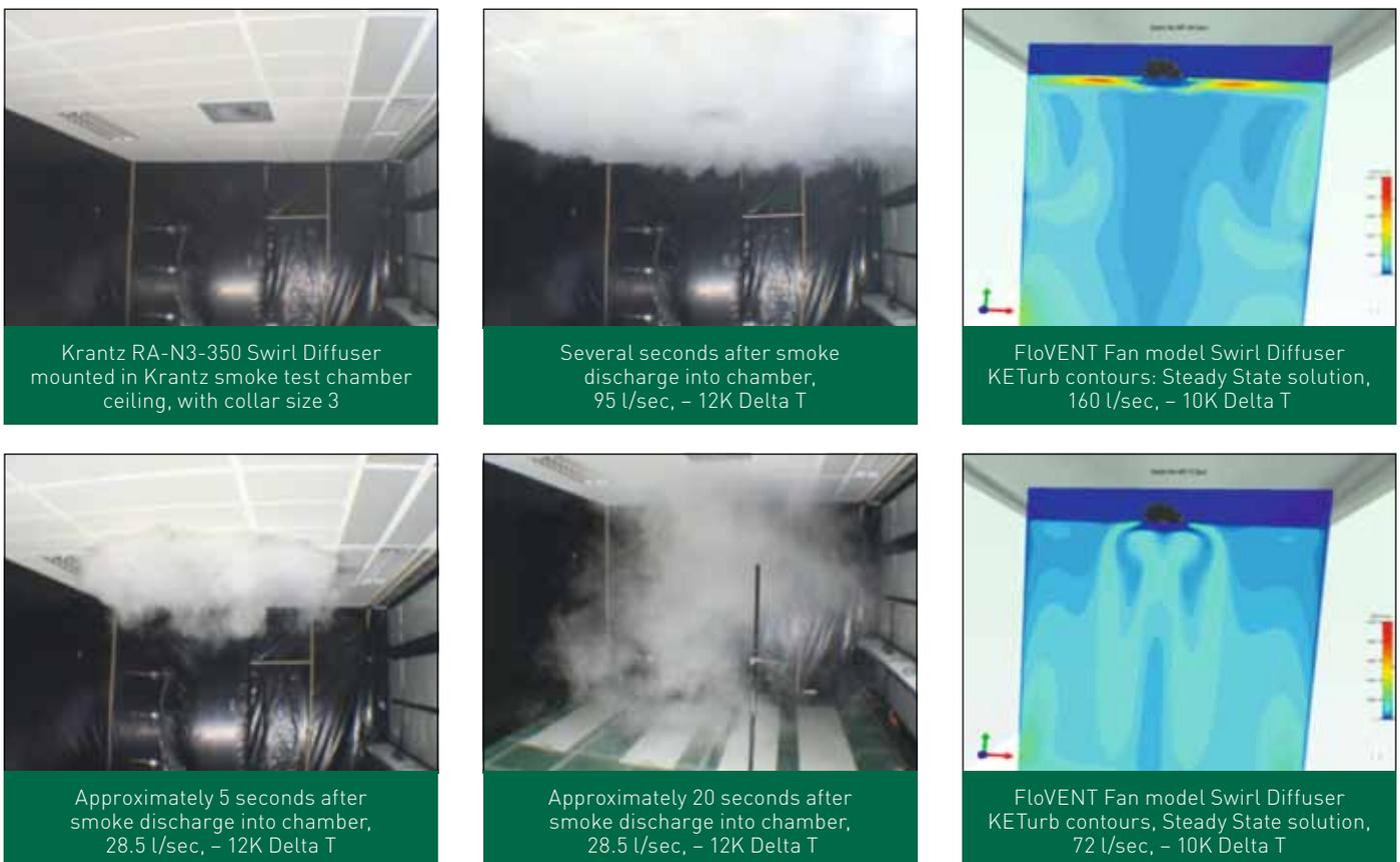
Figure 1: Selected images from Krantz video footage of Swirl diffuser smoke test performance, compared with KE Turbulence plots of the FloVENT fan model swirl diffuser at nominal flow and at 45% turndown.
