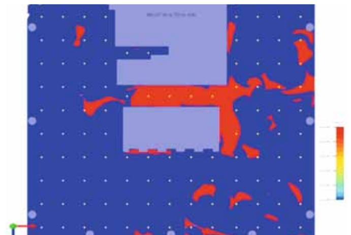
Figure 8: ACE at 1000mm height at maximum flow rates, with slots removed
